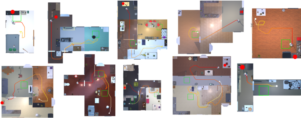
Figure 4: Top-down views across indoor environments with SafeDec induced trajectories Red circles mark target objects, green boxes are avoid regions, and orange paths show safe trajectories under constrained decoding.
